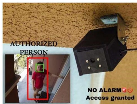
Figure 1: Illustrates when the person's face is identified, the doors will open and the lights will turn on.
