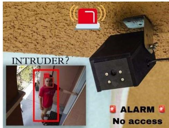
Figure 2: Illustrates an intruder alarm will be triggered along with the denial of access.
